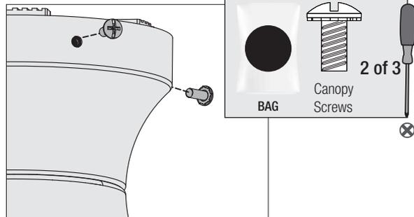
Hold the canopy up with the screw holes aligned. Partially install two canopy screws, found in the ● hardware bag, into the holes opposite the ceiling plate hooks.
