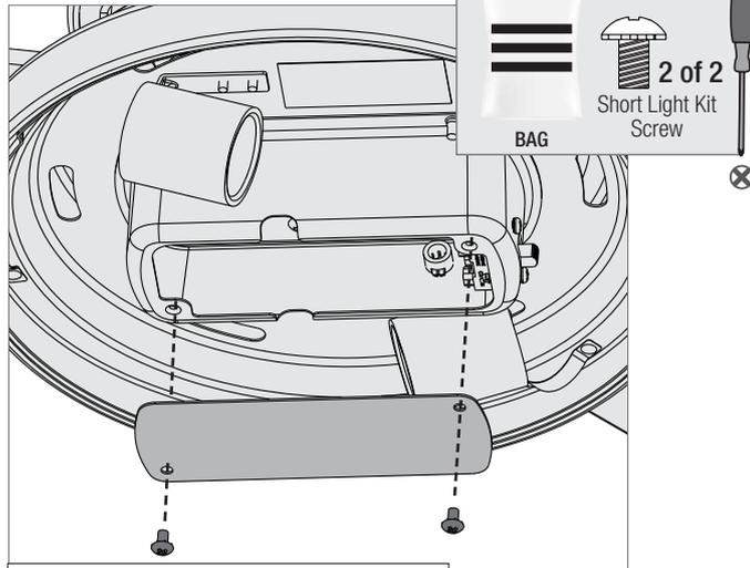
Carefully push all switch housing components into the switch housing, then install the switch housing plate using two short light kit assembly screws, found in the hardware bag.
