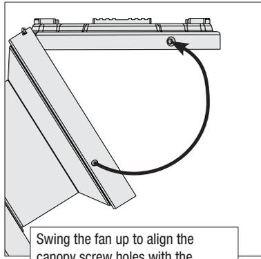
Swing the fan up to align the canopy screw holes with the mounting holes on the ceiling plate.
