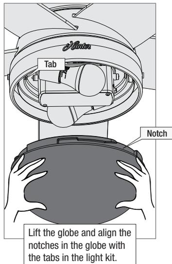
Lift the globe and align the notches in the globe with the tabs in the light kit.
