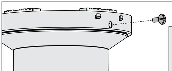
Partially install a canopy screw, found in the ● hardware bag, between the ceiling plate hooks. When all the holes are properly aligned, securely tighten all three canopy screws.
