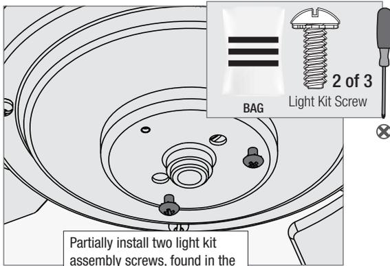
Partially install two light kit assembly screws, found in the hardware bag, halfway into the motor housing as shown. It does not matter which two screw holes you choose.
