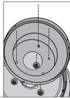
Place the canopy on the top housing. Ensure all four screw holes line up with the screw holes in both the top housing and the canopy.
