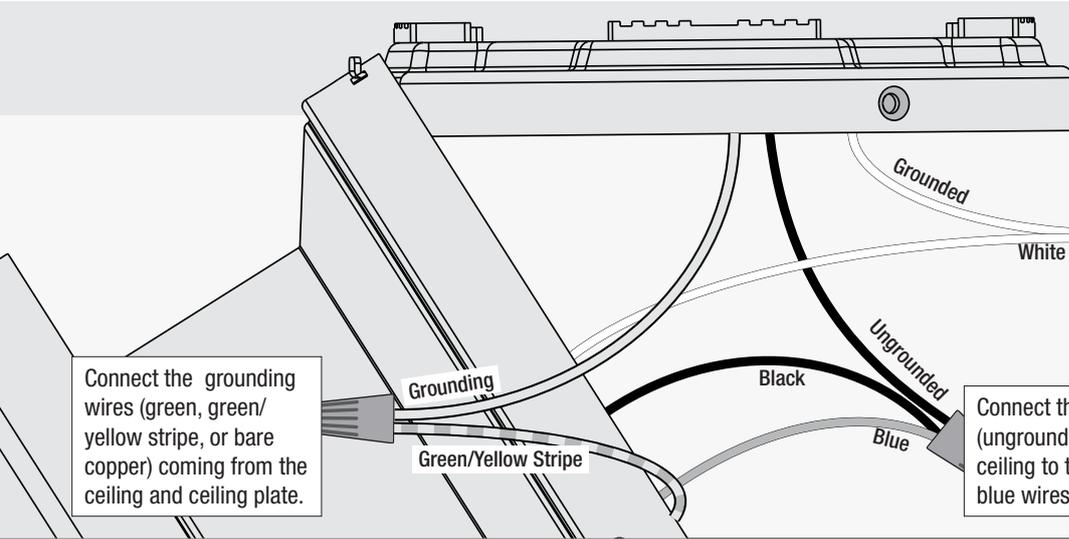
Connect the white (grounded) wire from the ceiling to the white wire from the fan.
