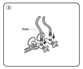
3. Connect the hose to the water supply pipe with hot water on the left and cold water on the right.
