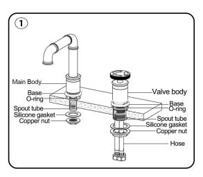
1. Install the 3 water inlet hoses on the switch valve together, install the base and O-ring, and then install the lock nut on the basin.
