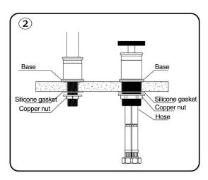
2. Tighten the nut, screw a water distribution pipe to the water distribution body and lock it.
