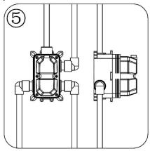
7. As shown in the figure, the leakage embedded box shall be removed, and the subsequent installation of control valve can be carried out after the wall room is laid
