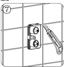
8. The notch of the upper hand wheel shall be inserted straight to the bottom, and the screw and hand wheel button shall be tightened; The lower hand wheel button is facing up, and the whole hand wheel is pressed to the end. When you hear the sound, you can finish it.
