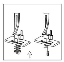
4. Re-install the rubber washer followed by the metal washer and lock-nut. Hand tighten then tighten further using a screw driver to tighten lock-nut screws.
