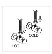
5. Attach flexible hose to water supply.
