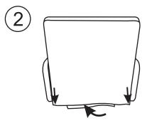
Smooth the flap down cover on back side, carefully match the velcro belt and press to secure.
