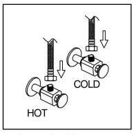
5. Attach flexible hose to water supply.
