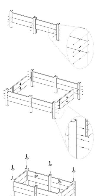
Using 2" screws, screw together the planter bed side. Be sure all parts are fully inserted into the posts before screwing.
