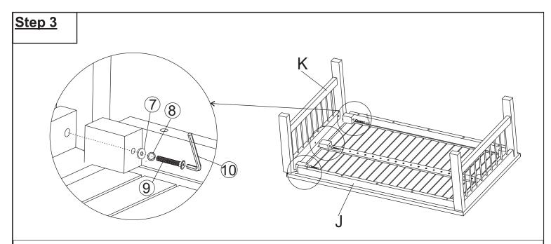
Repeat the same process of step 2 to attach attach Leg Panel (K) to the Table Top (J) using 3 Washers (7), Spring Washers (8), Bolts (9) with Allen Wrench (10)
