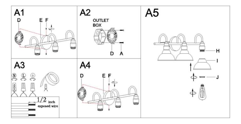
Step A1: Unscrew studs (F) from back plate (E), then set them aside for later installation.
