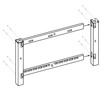
Insert one 51½" table rail (part 5) into 38" front right post (part 4). Insert one 51½" shelf rail (part 6) into 38" front right post. Insert free ends of table and shelf rail into 38" back left post (part 3). Using four ¾" screws per post, screw together potting bench front panel. Be sure all parts are fully inserted into posts before securing. Using included super glue tube, glue 4" sq. flat post cap (part 16) onto top of each post.
