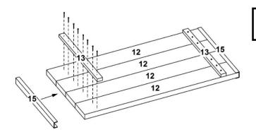
Lay out four 43" table top rails (part 12) with pilot holes facing up. Set each 22" table top brace (part 13) over pilot holes of table top rails. Using eight 1¼" screws per table top brace, fasten table top braces to table top rails. Apply glue to inside edges of 22" table top end cap (part 15). Press end cap onto ends of table top (DO NOT slide from end). Take care that end cap is flush with ends of table top and use a file to round off any sharp edges.
