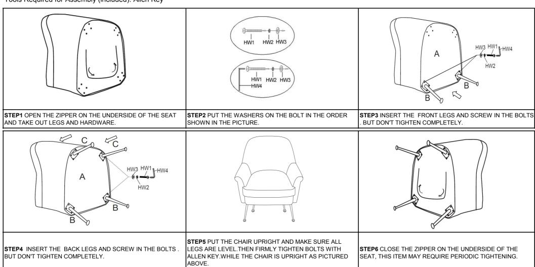
The legs and hardware are located in the small box underneath the chair in the zipper compartment.
