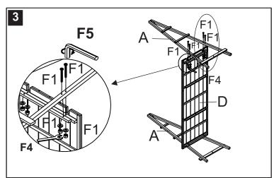
Step 3: attach the leg (A) to the other side of table top (D) as shown on the picture .Repeat assembly same step 2.
