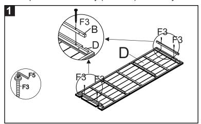
Step 1: attach connection bar (B) to the table top (D). Using the allen screw S (F3) and tighten with the Allen key (F5) as shown on the picture. Both side are same.
