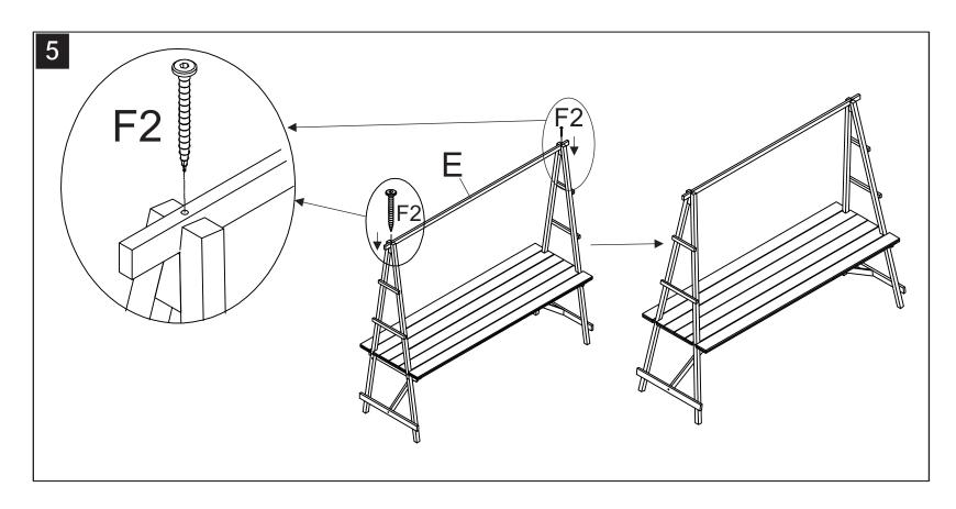
Step 5 : put the top bar (E) on top the leg (A) as shown on the picture. Tighten the Allen screw L (F2) with the Allen Key (F5).
