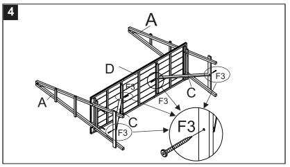
Step 4: put the support bar (C) under table as shown on the picture. Using the Allen screw S (F3) and tighten with the Allen key (F5).
