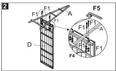
Step 2: attach the leg (A) to the table top (D) as shown on the picture. Using the allen bolt (F1) and tighten with the wrench (F4) and the allen key (F5).
