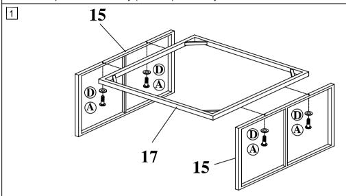
Step 1 Connect Stool Side Frame (15) & Stool Top Frame (17) & tighten Bolt (A) with Allen key (E)
