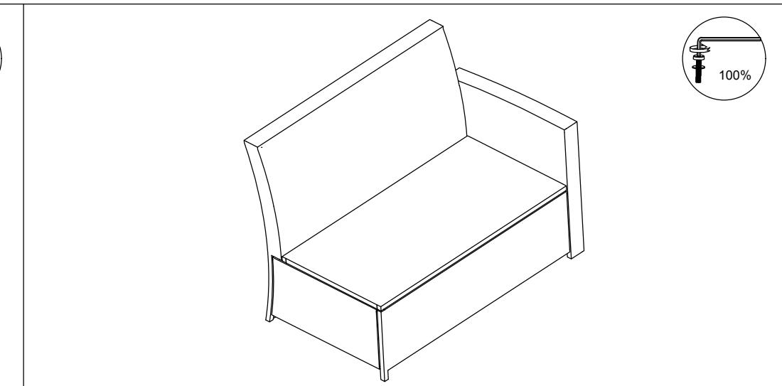
STEP 6: Put the Left Bench upright and make sure all legs are level, then firmly tighten Bolts with Allen Key (HW6).
