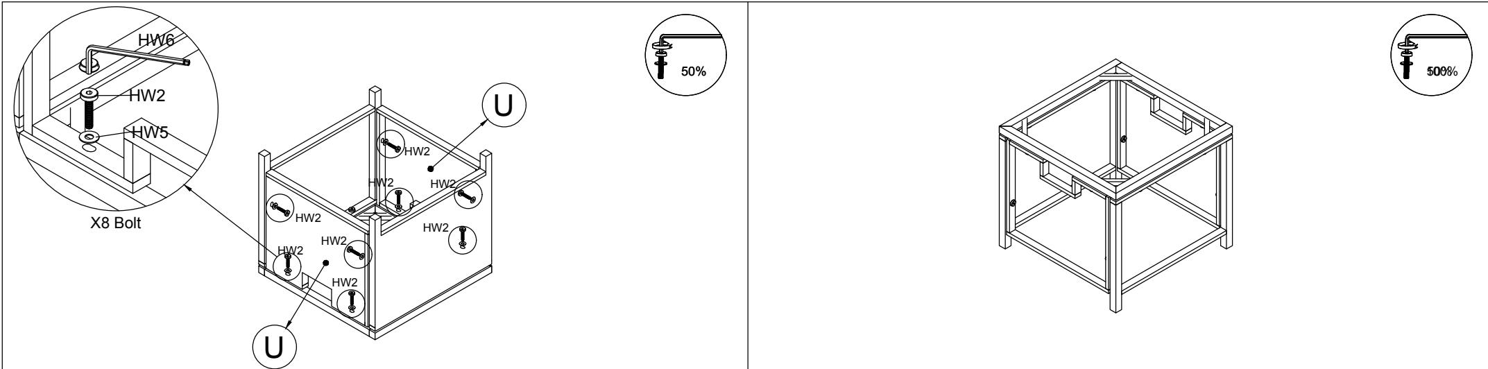
STEP 9: Connect the Part from STEP8 and Stool Front/Side Frame (U), tighten Bolt (HW2), Flat Washer (HW5) with Allen Key (HW6)
