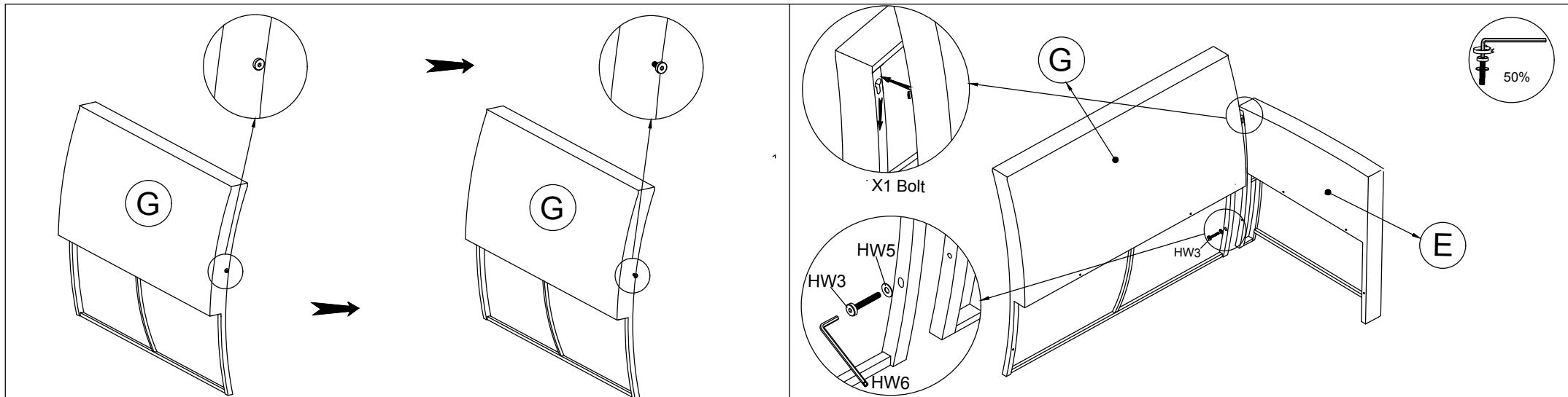
Step 1: Use Allen Key to loosen Bolt on the side of Right Back Frame (G) about 10 mm.
