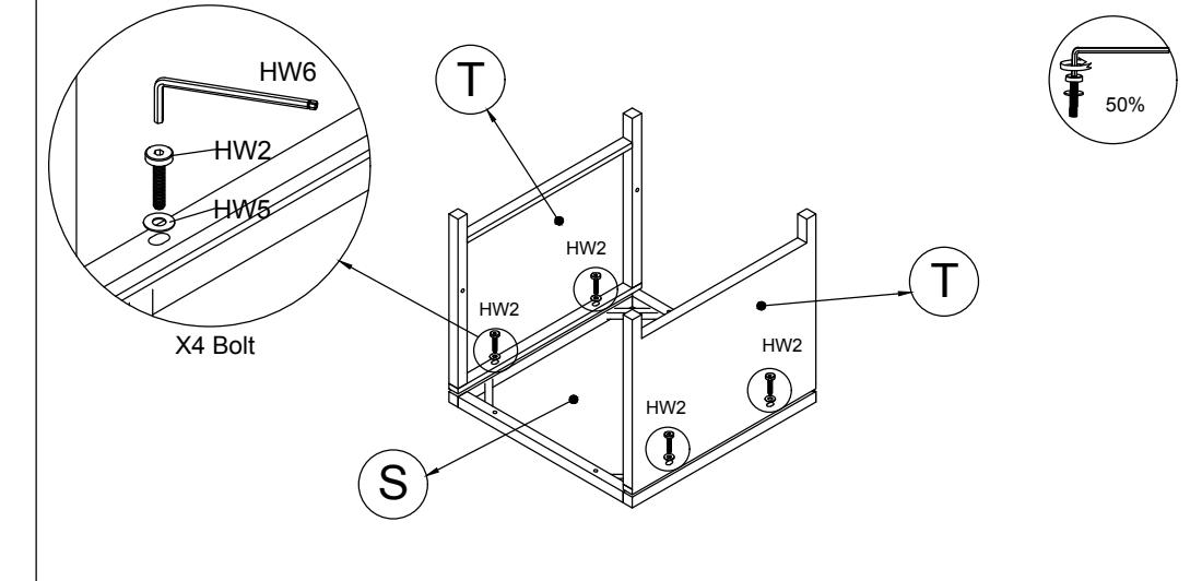
STEP 8: Connect The Stool Seat Frame (S) & Stool Leg Frame (T), tighten Bolt (HW2), Flat Washer (HW5) with Allen Key (HW6).
