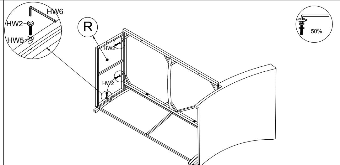
STEP 4: Connect the Part from STEP 3 and Corner Side Frame (R), tighten Bolt (HW2), Flat Washer (HW5) with Allen Key (HW6).
