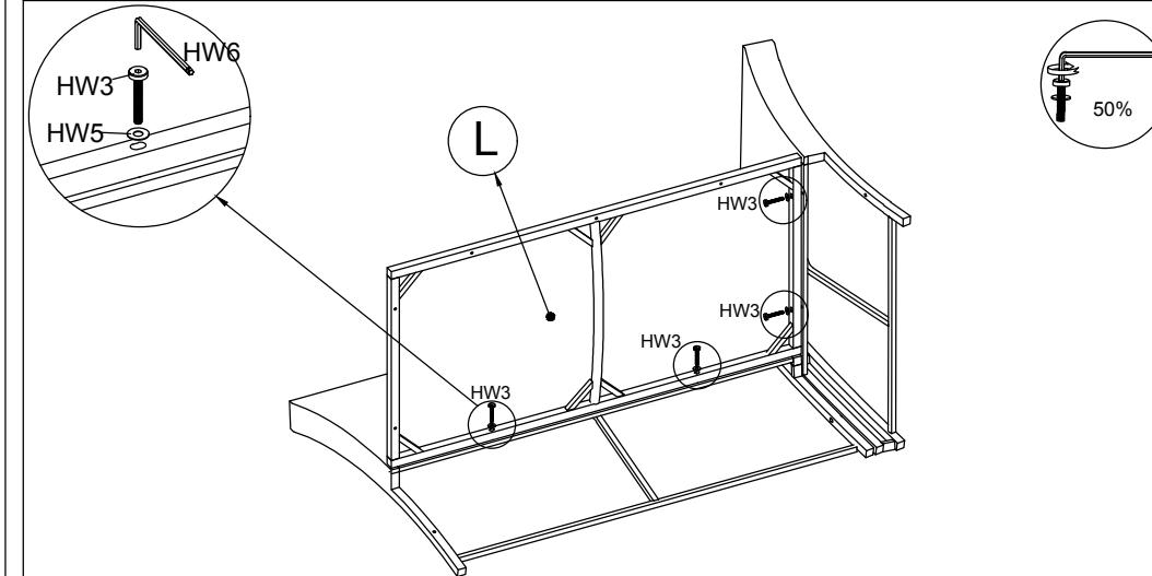
STEP 3: Connect the Part from STEP 2 and Corner Seat Frame (L), tighten Bolt (HW3), Flat Washer (HW5) with Allen key (HW6).
