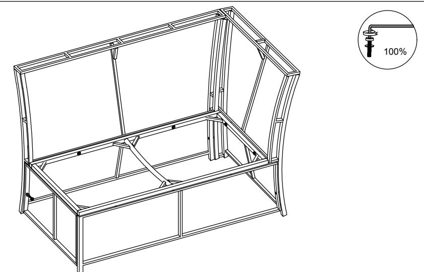
STEP 6: Put the Corner Bench upright and make sure all legs are level, then firmly tighten Bolts with Allen Key (HW6).
