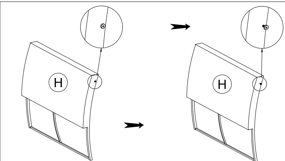
Step 1: Use Allen key to loosen Bolt on the side of Corner Back Frame (H) about 10 mm.
