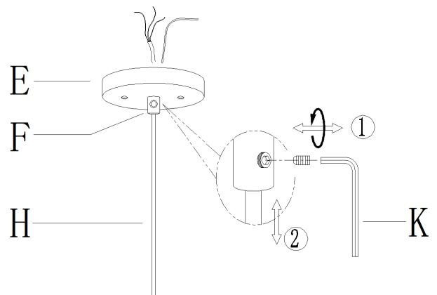
5. If needed, shorten the extra length of the fixture wires from cord (H) so that they all are at least 6 inches (152.4 mm) long above canopy (E) within the outlet box.
