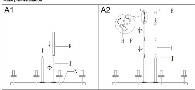
Step A1: Screw the threaded pipes (J) onto the iron frame (N), then place the square iron pipes (K) on threaded pipes (J).
