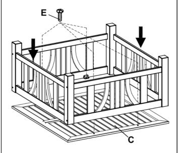
Put the table top (C) face down on a clean flat surface. Put the pre-assembled side frames into table top (C) and secure the metal clips using 1/2" bolts (E).
