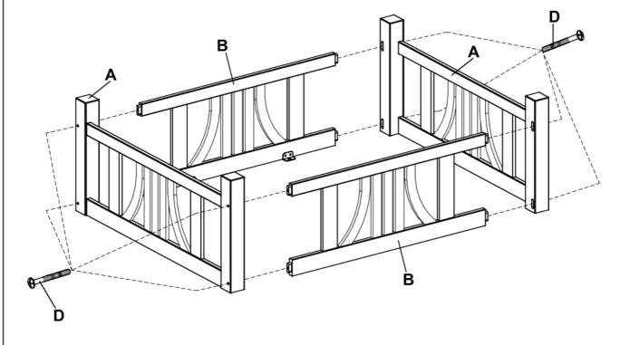
Attach side frame (A) into side frame with metal clip (B) as shown. Secure using 2 1/4" bolts (D) and tighten all bolts using screwdriver.
