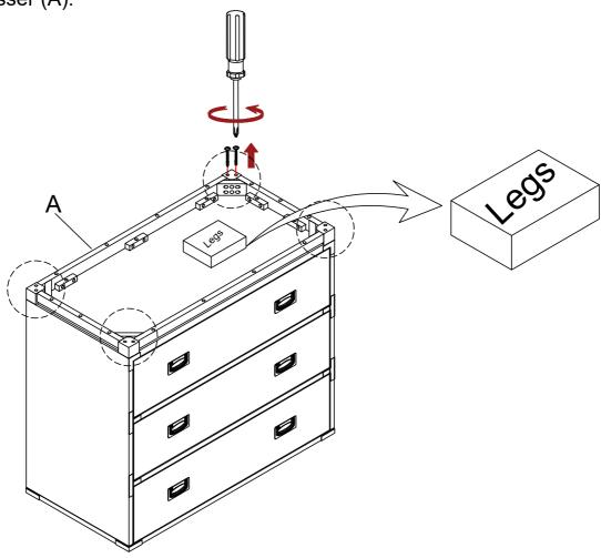
2 Attach the Leg (B) to the Dresser (A) using Allen Bolt (C), Lock Washer (D) and Flat Washer (E) with the Allen Key (F).
