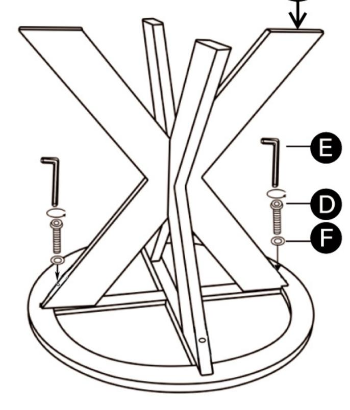
Attach wooden leg "C" to bottom of table top by bolts and flat washers.
