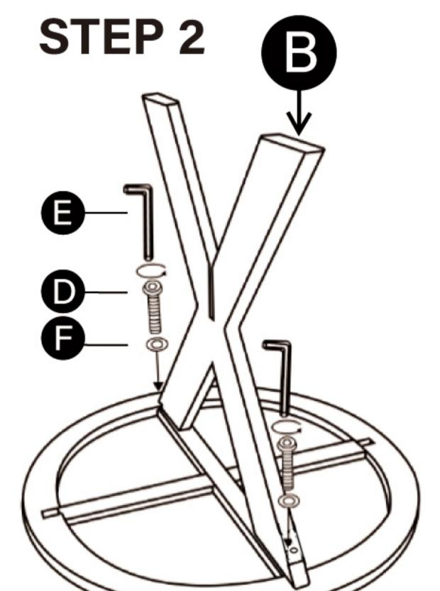
Attach wooden leg "B" to the bottom of the table top by bolts and flat washers as shown above.
