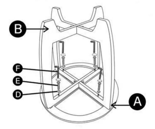
Put the table top upside down. Open wood base, attach wood base to table top by bolts and flat washers asshown above.
