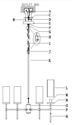
Step A1: Screw the stems (Q) to the bottom of the arms (P).
