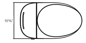
This toilet is designed to rough-in at a minimum dimension of (12") from finished wall to C/L of outlet. Supply not included with fixture and must be ordered separately.
