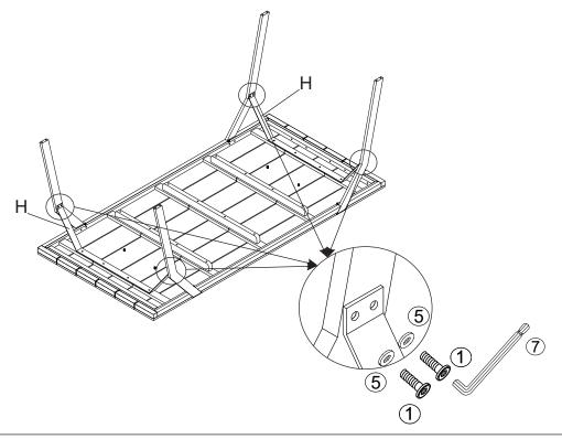
Attach the Connector Bar (H) to the First Leg (F) and Second Leg (G) using Bolts (1) and Washers (5) with the Allen Wrench (7) as shown above. **Do not fully tighten the Bolts.**
