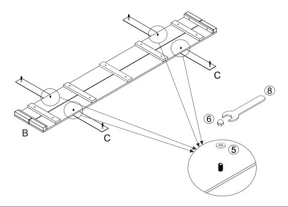
Place Bar (C) facing down on a clean, non - marring surface. With the help of your adult partner, position the Middle Table Top (B) to the Bar (C) using Cap Nuts (6) and Washers (5) with the Wrench (8) as shown above. **Do not fully tighten the Cap Nut.**
