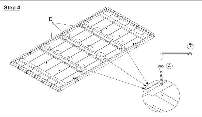
Attach the First Support Bar (D) to the Side Table Top (A) and Middle Table Top (B) using Screws (4) with the Allen Wrench ( $\overline{\mathcal{T}}$ ) as shown above **Do not fully tighten the Screws**.
