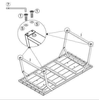
Attach Support Leg (I) to the First Leg (F) and Second Leg (G) using Bolts (1) and Washers (5) with the Allen Wrench (7) as shown above. **Do not fully tighten the Bolts.**
