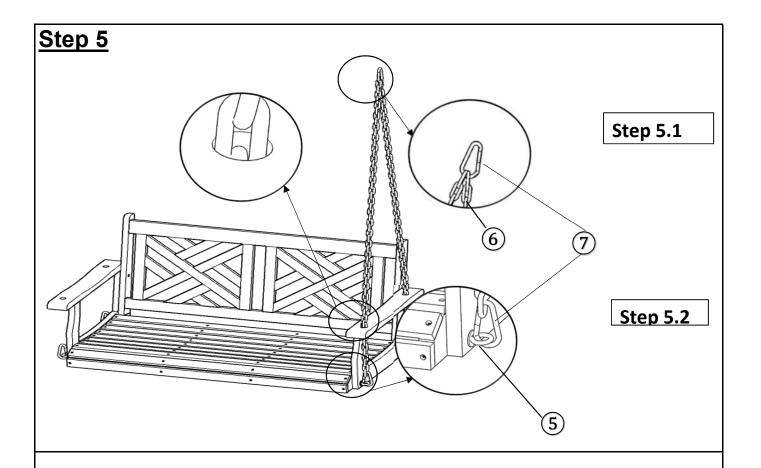
**Step 5.1:** Unscrew the connection on the Carabiner (7), then loop the Chain (6) onto the Carabiner (7), and screw the connection shut as shown above.
