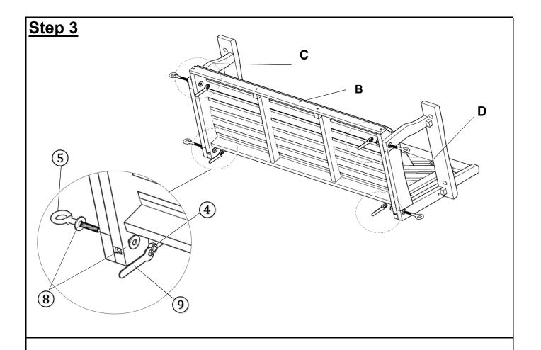
Insert the tenons of the Seat Panel (B) into the mortises of the Left Arm Panel (C) and the Right Arm Panel (D), then attach all three parts by using Lock Nuts (4), Washers (8), and Eye Bolts (5), with the Wrench (9) as shown above.
