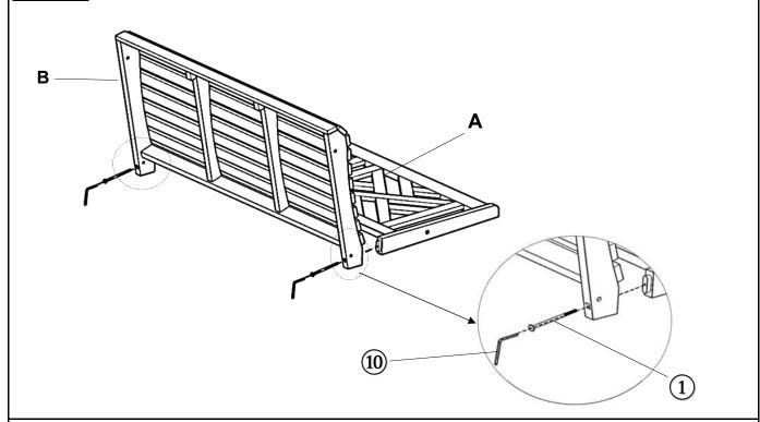
With the assistance from your adult partner, attach the Backrest Panel (A) to the Seat Panel (B) using Screws (1) and the Allen Wrench (10) as shown above. **Do not fully tighten the Screws.**
