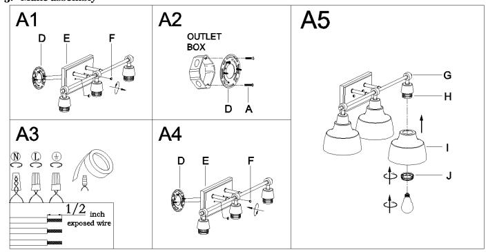
Step A1: Unscrew the ball knobs (F) from the back plate(E) then gently remove the mounting plate (D).
