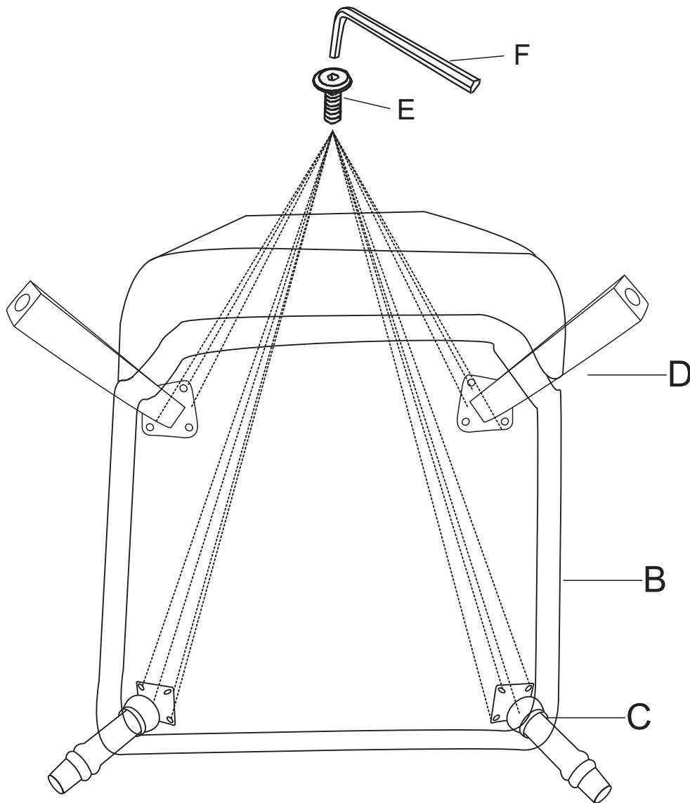
**STEP 3 :** Use bolt E, allen key F to connect the leg C/D to bottom of the seat cushion B, make sure all holes align, fasten all bolts to secure.
