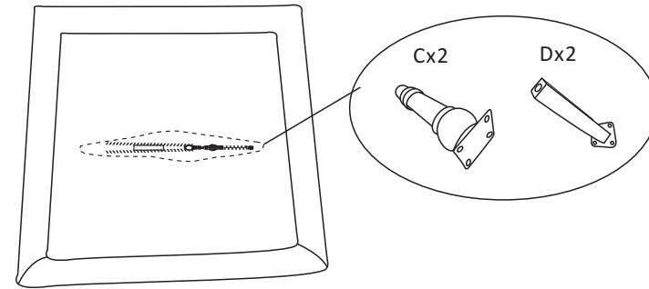
**STEP 1:** Open the zipper pocket under the seat and take the legs C,D out.
