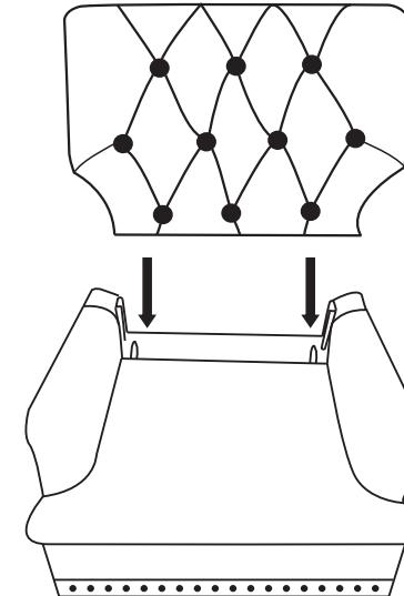
**STEP 2:** Carefully align male and female bracket then push the back all the way down to secure.
