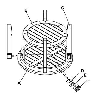
Attach the tray (B) to the legs (C). Attach the other legs (C) into the table top (A) and tray (B), as diagram shown.
