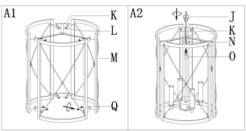
Step A1: Fix flat iron stent (K) and flat iron bars (Q) to iron frame (M) with screws (L).
