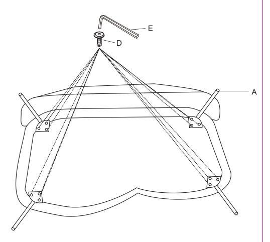
**STEP 2:** Use bolt D, allen key E to connect the metal leg B to bottom of the seat cushion A, make sure all holes algin, fasten all bolts to secure.
