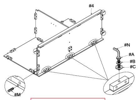
Align panel (#4) to the unit, then secure by using bolts (#A) with washers (#B,C). Insert dowels (#M) to panel (#4).
