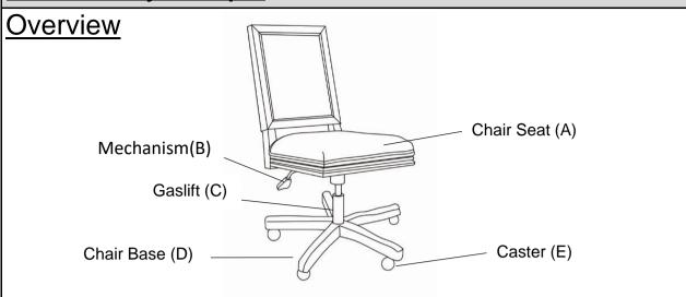
This Office Chair has multiple parts and may require up to 30 minutes to assemble. To give you an overview of the Office Chair parts, the above picture is to help you put the various parts into perspective. Please read through the instructions below to familiarise yourself with the parts and steps before assembly.
