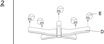
Insert the Casters (E) into the mounting positions of the Chair Base (D) as shown above.
