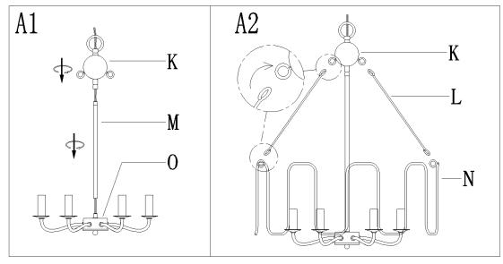
Step A1: Screw the stem (M) onto the iron ball (K) and then screw stem (M) onto the arms assembly (O).
