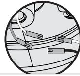
Feed the wires coming from the bottom of the motor housing through the center hole in the light kit assembly. Connect the wires from the fan. Connect the white wire to the white wire. Connect the blue wire to the black wire. Tuck the excess wiring above the light kit.
