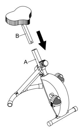
Adjust Seat Post (B) to suit for your height, then fasten with Fix Bolt (L) as below shown.
