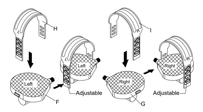
Assemble Pedal-Left (F) and Pedal-Right (G) to Bike Main Body (A), then fasten by Spanner (O) as below shown.
