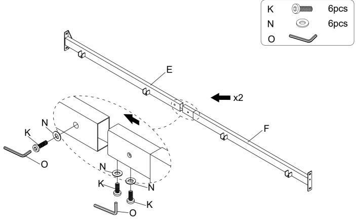
Assemble the pre-connected Side Rail - Front (E) & Side Rail - Rear (F) to Extension Leg - Left (C) & Extension Leg - Right (D) and Footboard (B), using Bolt (K), Bolt (M) & Flat Washer (N) by Allen Key (O) with Hex Nut (P) by
