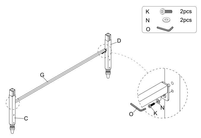
Assemble Headboard (A) to Extension Leg - Left (C) & Extension Leg - Right (D), using Bolt (K) & Flat Washer (N) by Allen Key (O).
