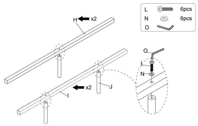
Attach the pre-assembled Slat - Middle (I) and Slat - Front / Rear (H) to Side Rail - Front (E) & Side Rail - Rear (F), using Bolt (K) & Flat Washer (N) by Allen Key (O) as below shown. K
