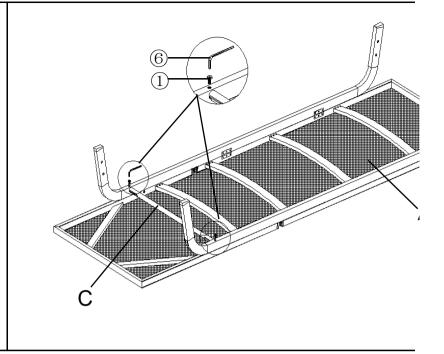
Open the carton and place all parts on a clean, undamaged suthe support bar(C) into the leg bars and affix it with bolts (1) a Key (6).
