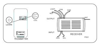
If there are two or more ceiling fans installed in the same house, in order to prevent your ceiling fans from being affected by the remote control of the adjacent ceiling fans, first turn the switch in each remote control transmitter to the CODE(locked) position (see the schematic diagram FIG1) Remarks: The standard state of the transmitter is in the common code COM
