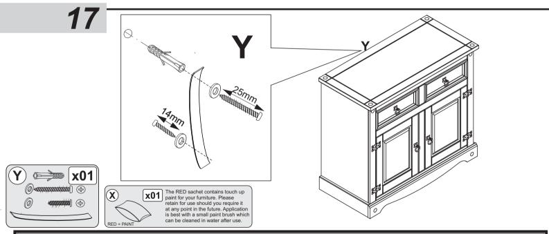
WARNING: CHECK FOR HIDDEN PIPES AND CABLES BEFORE DRILLING.
