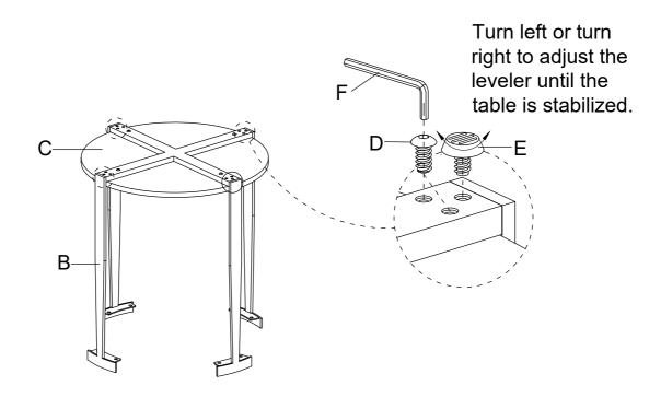
Assemble Leg Post (B) to Table Top (A), using Bolt (D) by Allen Key (F) as below shown.
