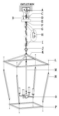
Step A1: Slip stem (M) over the wires and then thread it onto the top of fixture loop assembly (O).
