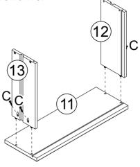
Attach part (12) and (13) in the part (15) using screw (C) and Phillips head screwdriver.
