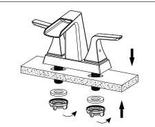
1. Please confirm the two holes on the basin are through holes as shown from the instructions before install.First,remove all fixing sets from the fixed group, and then put the body through the hole on the basin, assemble all fixing sets to the body.
