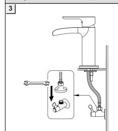
3.Connect the inlet hose from the body,"Red" for connecting to the hot water, and "Blue" for connecting to the cold water.
