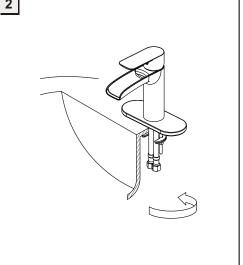
2.According the remove step to screw up the fixing set to the mixer below the basin. Use hand to screw up the locknut, then use install tool for fixing strengthen.
