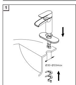
1.Make sure there is a Ø30-Ø33 Hole on the basin before fix the mixer, Unscrew the fitting ASSY from the bottom of the body, then get the body through the hole, don't forget to fix the o-ring between the bottom of the body and the basin.
