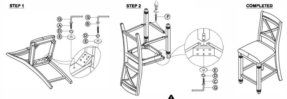
(1) Align the seat to the chair back, insert the bolt and washer to pre-drilled holes and tighten it. (2) Attach side stretcher to chair back then attach front legs (L & R) to side stretchers (L & R) and seat cushion, insert the nut and washer then tighten front chair to cushion seat. Insert screws to stretcher then tighten by using screwdriver (not provide).
