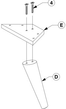
Bolt the Post & Support Panel (D & E) to the Side Rail (C).
