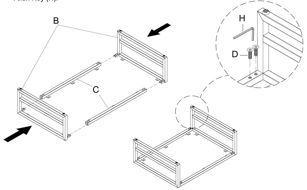
Attach Leg Frame and Metal Bar Assembly (B & C) to the bottom of Cabinet (A) by using Allen Bolt (E), Lock Washer (F) and Flat Washer (G) and tighten with Allen Key (H).
