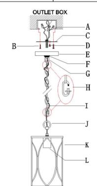
Step A1: By measuring, determine the correct number of links needed for proper hanging height. Using the chain pliers, disconnect and discard the unwanted part.
