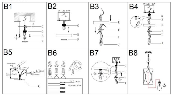
Step B1: Remove the collar ring (F) from collar loop (G). Attach the single bar (C) to outlet box with mounting screws (B).
