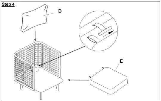
Stand the assembled part in Step 3 up, then put the Seat cushion (E) and the Back cushion (D) on the Chair
