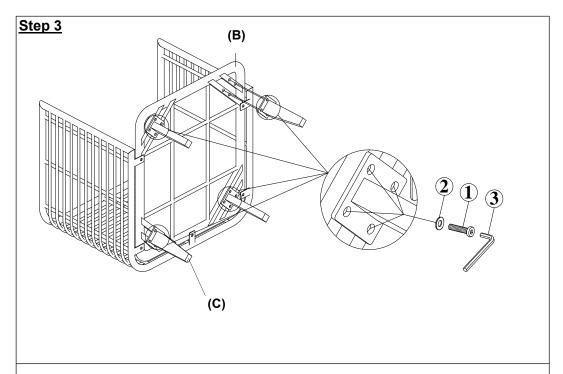
With the help from your adult partner, attach all the Legs (C) to the Seat Panel (B) of the assembled part in step 2 by using the Bolts 1, Washers 2 and the Allen Wrench 3 as shown in the picture above
