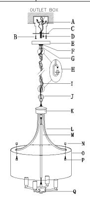
Step A1: Slip stem (M) over the wires and then thread it into the top of lower fixture loop assembly (Q).
